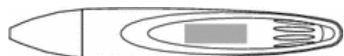
Screen print, On the inner barrel, writing position, back side Dimensions: 26x6 mm - max. colours: 2 Tampo print, On the inner barrel, writing position, back side Dimensions: 22x7 mm - max. colours: 4
